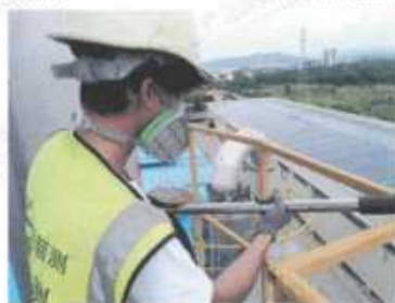
DA008 动态反应器废气排放口废气采样
